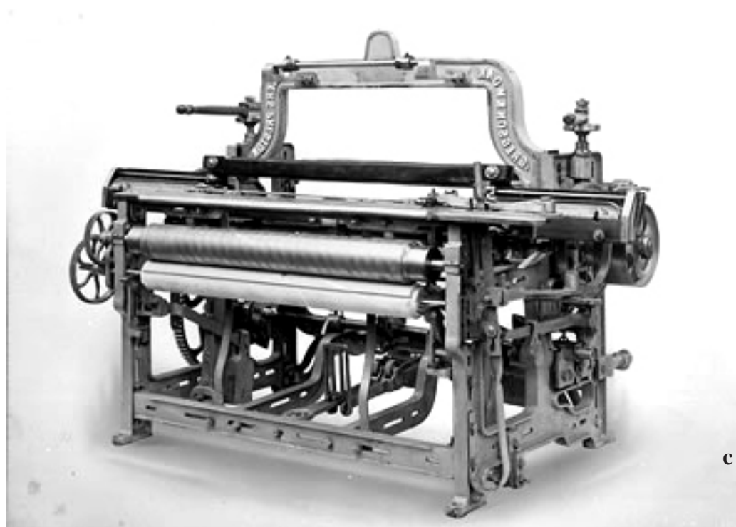
a) James Hargreaves' Spinning Jenny, b&c) Edmund Cartwright's Power Loom
