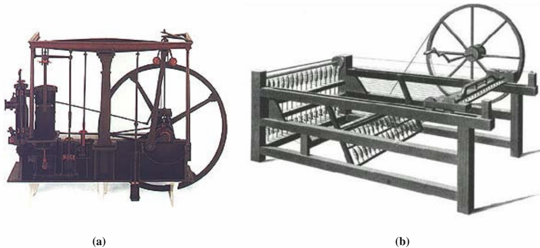
Fig.12.6: The a) steam engine and b) spinning jenny that powered the Industrial Revolution
