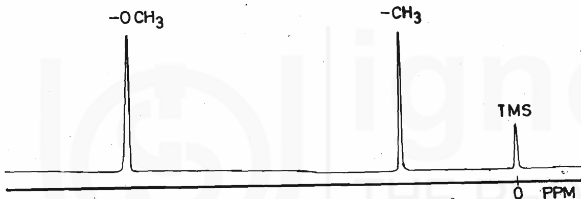
Fig. 10.9: The NMR spectrum of methyl acetate (not drawn to scale) showing two peaks from the two chemically different methyl groups and the TMS at 0 ppm.
