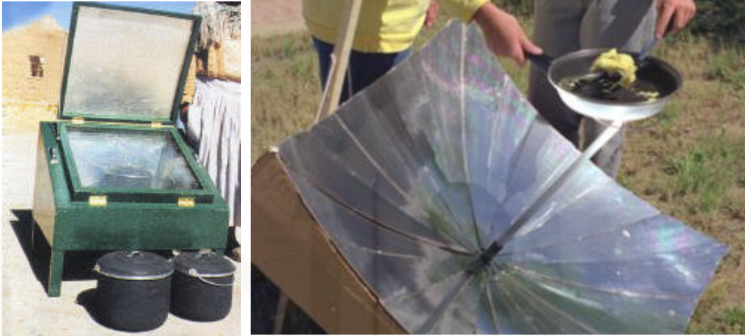
Fig.13.4: Solar cookers: box type and one that uses a reflector
