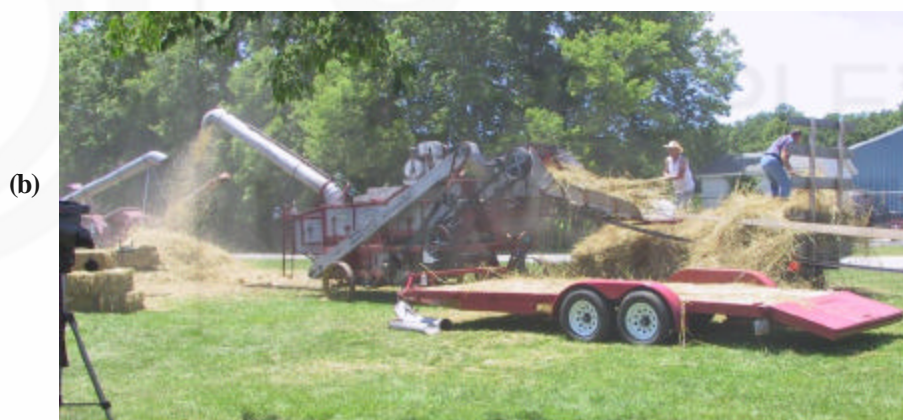
Fig.10.7: a) Harvesting combine; b) thresher
